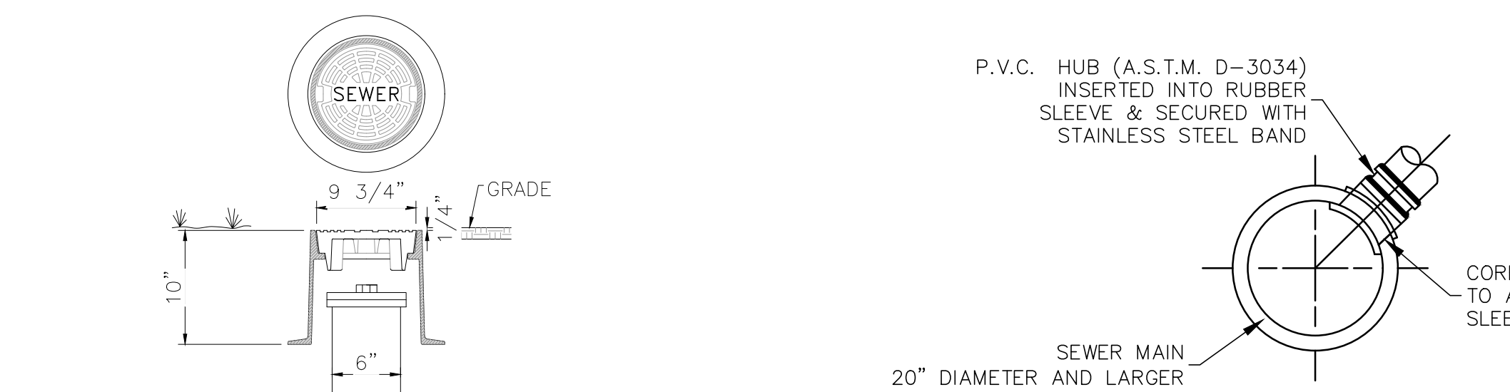
Cast Iron Cleanout Covers Not to Scale Inserta - Tee Not to Scale
